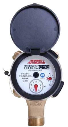
The D10 is a positive displacement meter that is suitable for use on potable drinking water systems. The meters have a low starting flow rate and excellent accuracy (+/- 1.5%) within the normal flow range.
