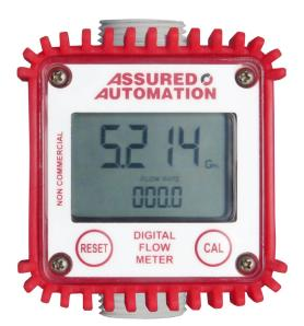
The DM-P Series multipurpose liquid flow meters use a helical turbine mechanism to give accurate flow measurements of cold water. It is constructed of durable plastic which makes it economical and chemical resistant. This versatile flow meter displays the current flow rate and records the lifetime total and a resettable batch total.
