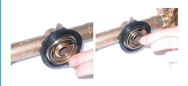
3. Position FAM Measuring Unit to Flow Tube; be sure the Measuring Unit is seated properly when mated with Flow Tube and that it is vertically level.
