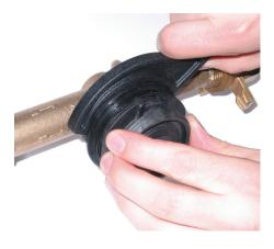
2. Replace both O-rings that are in the Flow Tube with new ones that were shipped with the FAM measuring Units. Apply a little lubricant on o-rings during this procedure.
