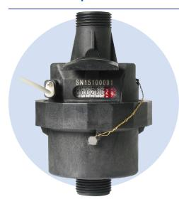
The WM-PD series water meters are volumetric piston displacement water meters. These meters use a mechanical transmission to advance a hermetically sealed, 8-digit register. They are suitable for use with potable cold water, and hot water. There are two sizes available, 1/2 inch and 3/4 inch.
