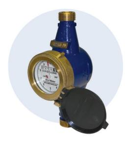
The WM Series water meters are multi-jet (inferential) impeller meters. They measure total flow in gallons. The impeller and magnet are the only moving parts in the measuring chamber. The chamber is located in a strainer basket, which allows for high amounts of impurities to be passed through the meter without affecting its operation. The impeller movement is transferred by a magnetic coupling to the hermetically sealed register.
