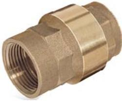
Lead free brass check valves are available to prevent reverse flow through meter. Reverse flow will deduct from the meter's total. The use of a check valve will also prevent the meter and upstream water from being contaminated by debris or additives like fertilizer that get added downstream from the meter.
