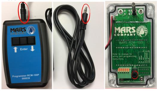
Connect one end of the 3.5mm jack into top of Programmer and the other end of the 3.5mm jack into the bottom center of circuit board.
