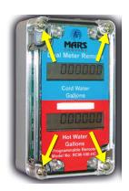
This exposes the back of the circuit board, where all the connections will be made. Also at this time, the rear of the casing can be mounted to the surface where the unit will be located via the two screw holes on the top left and bottom right of the casing.
